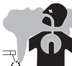
Fumes, gas and dust produced during welding are hazardous to health. It is mandatory to ensure adequate ventilation and/or extraction to keep fumes and gas away from the work area. Using an air fed welding helmet is recommended in case of insufficient ventilation in the workplace.
